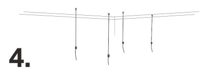
Screw assembled cables into the fixed ceiling mounts.
