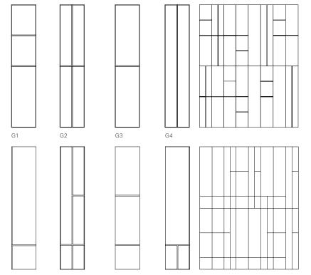
Standard Panel Size 3000m x 600mm x 75mm 3050m x 600mm x 75mm 3100m x 600mm x 75mm 3300m x 600mm x 75mm Also available in custom lengths.
