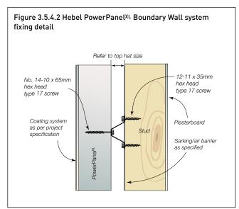
NOTE: When positioning the stud frames allow 5-7mm extra cavity width for the sheet bracing between top hat and timber stud.
