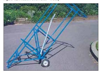
Figure 4.2.2 Hebel Hoist
