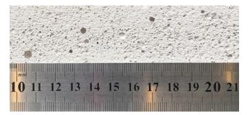
Cross section of AAC, showing the voids.
